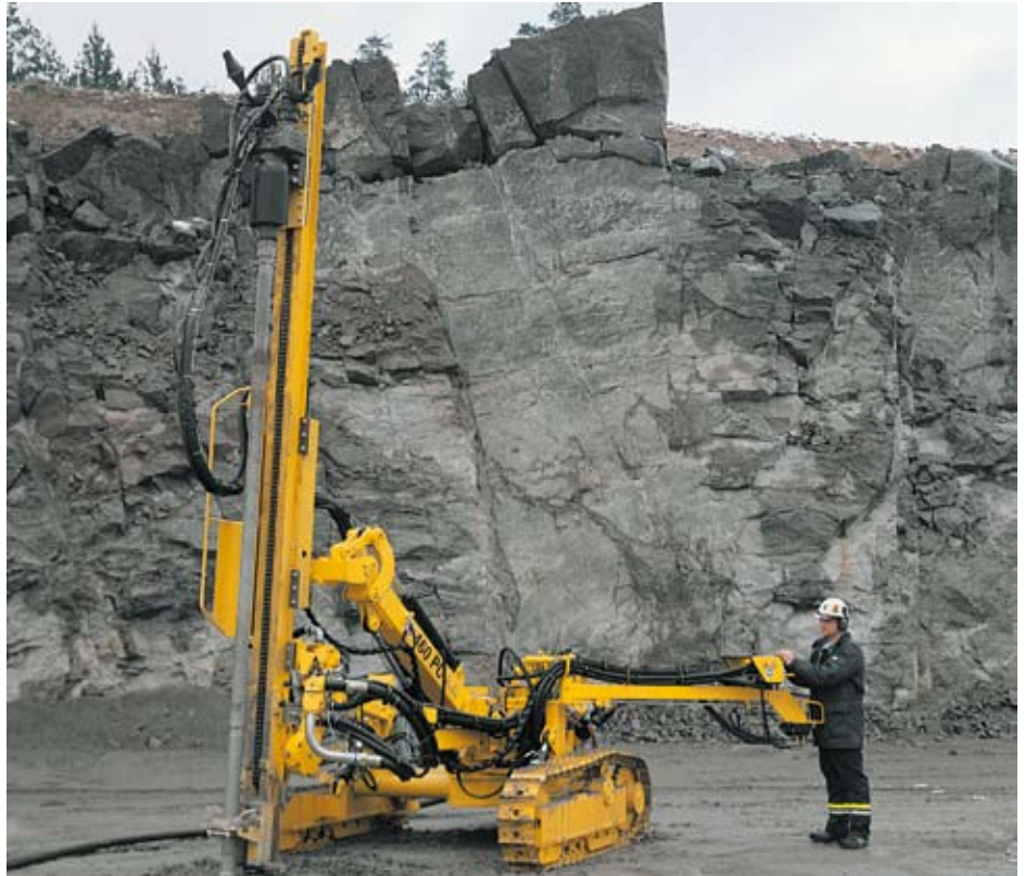
ROC 460 HF (heavy feed) equipped with reinforced feed beam is capable of drilling up to 6 1/2" holes down to 140 metres (459 ft)
